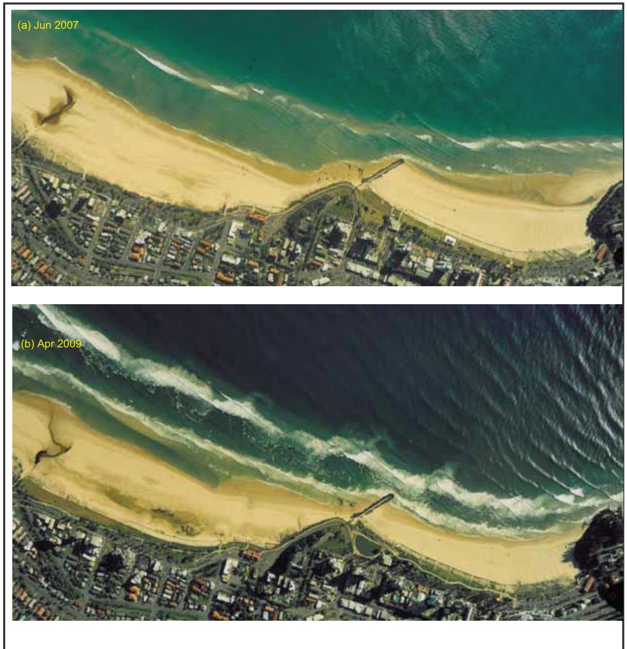
Figure 11 Sand movements post TRESBP 2007-2009
