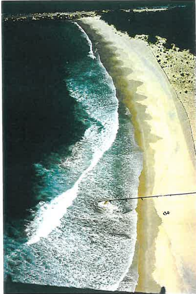
Plate 4 : Aerial view of the turbidity plume drifting north of the sand discharge. Note also the substantial turbidity generated by the breaking waves.
