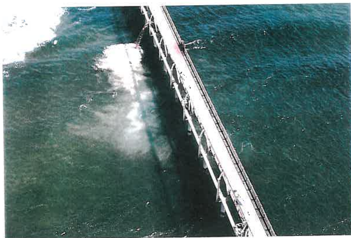
Plate 12 : Aerial view of plume, also showing marker float position of moored current meter.
