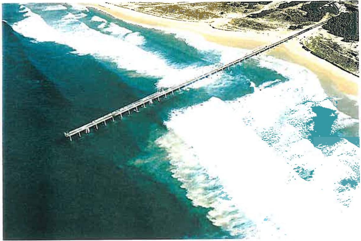
Plate 7 : Corresponding turbidity conditions adjoining the sand by-passing jetty at the Spit on the 22nd August, 1996. Note the large amount of wave induced turbidity.
